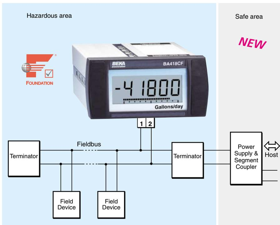
The **BA418CF Fieldbus Indicator** is a new cost-effective intrinsically safe panel mounting instrument that displays a single fieldbus process variable in a hazardous area. Housed in a robust panel mounting enclosure with an IP66 front, the instrument has a large, high contrast five digit display and a horizontal bargraph. The BA418CF indicator uses the same technology and compliments the well established BEKA eight variable fieldbus displays that are now in worldwide use.
