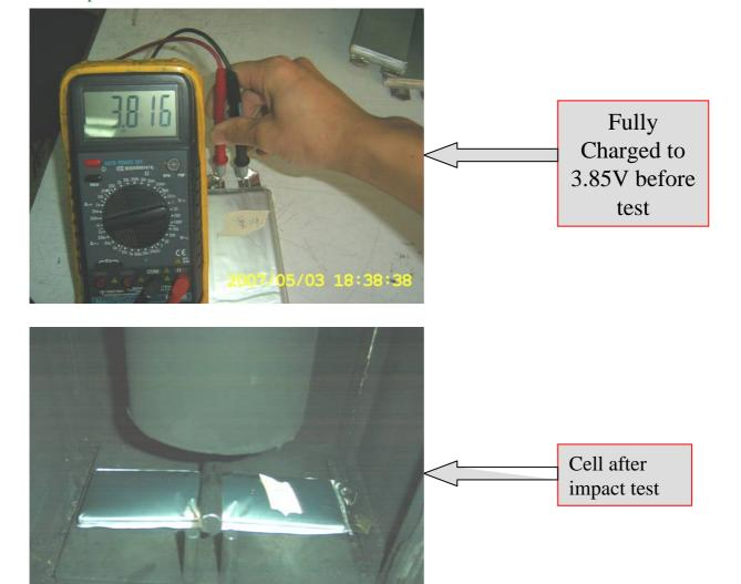
Result: No Explosion, No Fire after impact test.
