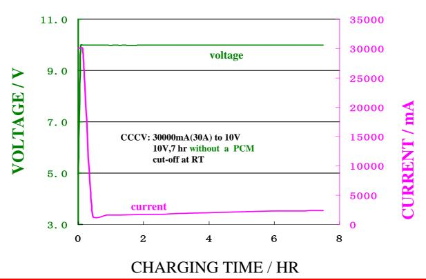
Results: The cell without PCM after 30A 10V overcharging test are no explosion, no fire.
