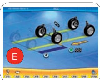
**(EN) «RUN-OUT» COMPENSATION PROGRAM:** Program to compensate «Run-Out» problems on tyre and rim and possible mistakes caused by an incorrect coupling between rim and self-centering clamp. The compensation value is calculated by pushing the vehicle for a distance corresponding to a wheel rotation of only 30°.
