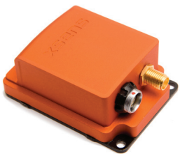
MTi-G encased: 57x42x23.5 mm, 55g 9-pins push-pull connector
