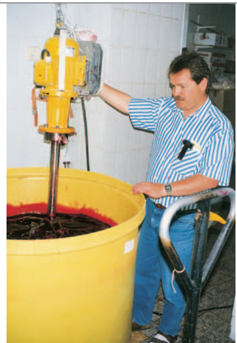
YTRON - Y HS on a Lift over an open Container Application: Dissolving of a Mix of various Minerals including Stabilizers
