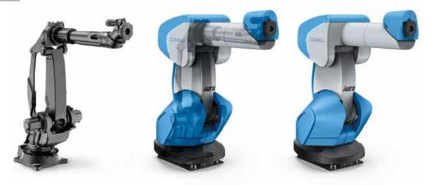
With AURA we transform a standard Comau Hollow Wrist robot into a collaborative solution.
