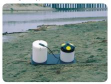
The Argonaut-XR on mounting plate with optional battery pack.
