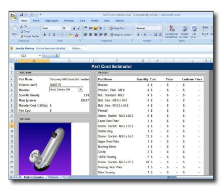
A cost estimator has leveraged the assembly tree directly from the CAD data to insert a complete parts listing into his estimate template. He has also embedded an interactive .3D file to visually clarify each part listed.
