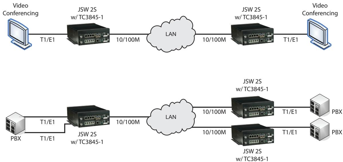
Typical Point-to-Point and Multi-Point Applications Using TC3845-1 to Extend T1/E1 Through an Existing Local Area Network
