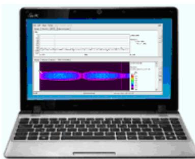
In **Spectrogram** mode ET 92 performs spectrum measurements in every second. The results are directly transferred to PC via USB port or indirectly by means of a memory stick when the measurement is completed.
