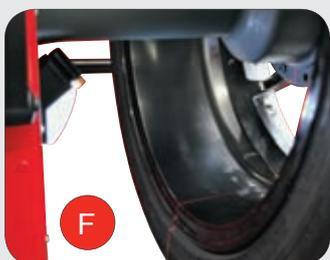
**(EN) VERSION TECO 68 PLUS L «LASER & LIGHT»:** Version complete with Laser line system and rim illuminator. If ALU programs are selected, the Laser line assists the operator during adhesive weight positioning at 6 o'clock. In this case the adhesive weight holder terminal of internal gauge will be supplied separately as standard accessory.
