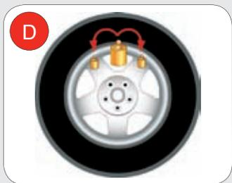
**(EN) HIDDEN WEIGHT AND SHIFT PLANE PROGRAMS (ALU P):** «Hidden Weight» subdivides the external adhesive weight in 2 parts to be positioned behind the spokes of the rim. The patented program «Shift Plane» calculates the balancing position to allow using commercial adhesive weights.
