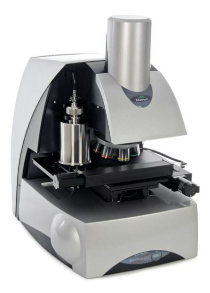
The Morphologi G3 measures the particle size and shape of dry powders, wet suspensions and particulates on filter membranes using the technique of automated static image analysis. The instrument is designed with the diverse needs of a multidisciplinary R&D lab in mind, while automation of analysis using SOPs makes it the ideal replacement for costly and time-consuming manual microscopy measurements.
