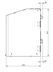
Material: Steel casing 3mm Width: 320mm Height: 515mm Depth: 375mm
