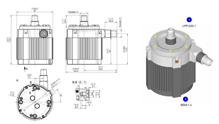
Figure 11: Dimensions of motor with pump head (dimensions in mm and [inch])
