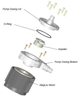
Figure 3: Disassembled pump head
