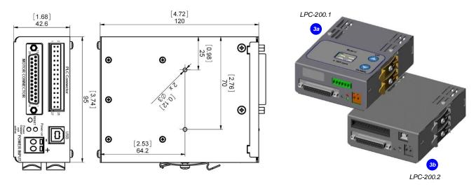
Figure 10: Dimensions of controllers LPC-200.2 (same basic dimensions for LPC-200.1)
