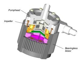
Figure 2: Maglev pump motor with pump head
