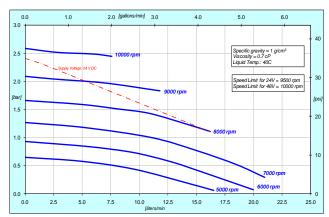
Figure 4: Pressure/flow curves for aqueous liquids (similar to water)
