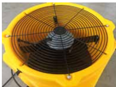
DFX 20 axial fan. The fan can be oriented in 8 different positions.
