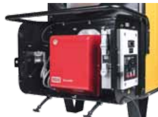
Into the box: Riello burner, digital control panel
