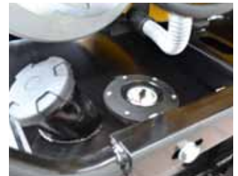
A leakless fuel tank closure and a big fuel level indicator.
