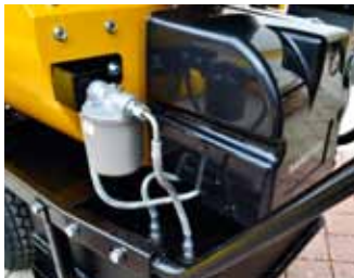
The heater gets the fuel from the tank below but can also be connected to an external tank. Fuel filter is outside. Fuel pre-heater is inside, within the combustion head.
