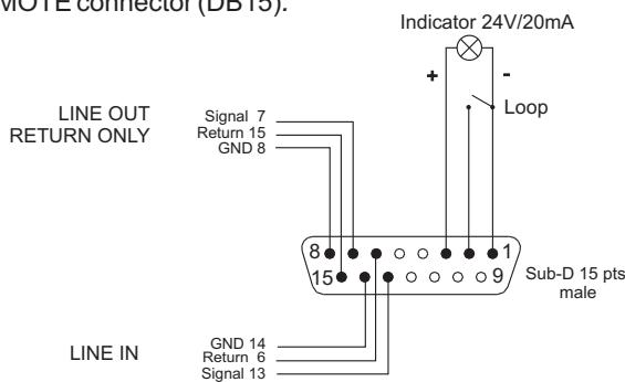
**Warning : Don't use in the same time XLR input/output and Sub-D 15 input/output.**
