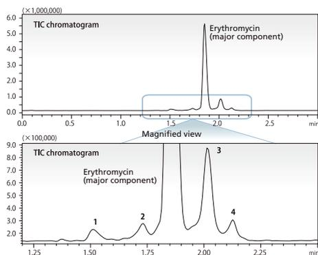
Using in-source CID allows the generation of fragment ions. This example shows the structure of impurities in erythromycin estimated from fragment ions generated by in-source CID. The multi-sequence mode permits several other methods within a single analysis, such as CID, positive/negative ion switching modes, and SCAN/SIM modes. Precisely setting the parameters reduces the risk of erroneous evaluations and enhances the reliability of analysis results.
