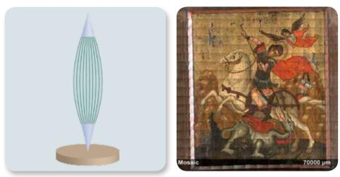
Diagram of the polycapillary optics used for X-ray beam focusing
