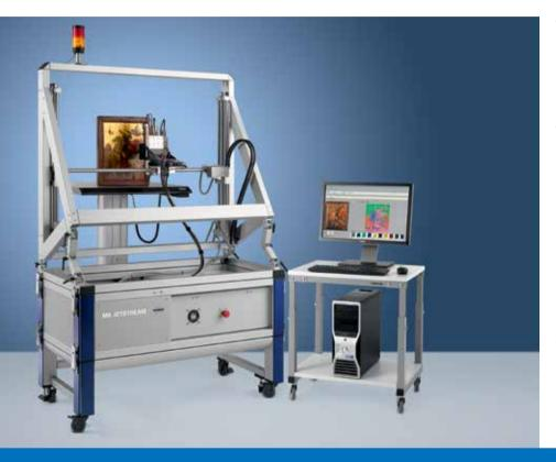
The Bruker M6 JETSTREAM is designed for the nondestructive elemental analysis of large samples. The mobility of the instrument allows it to be placed at the site of the object of interest, such as a gallery, museum or the shop floor. The performance parameters enable scanning areas of 800 mm x 600 mm with a variable spot size down to 100 µm and speeds of up to 100 mm/s.
