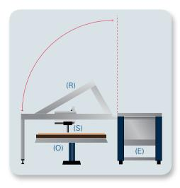
Diagram of the M6 JETSTREAM set-up in the horizontal measurement position, showing analysis object (O), spectrometer head (S), rig (R) and electronics compartment (E)
