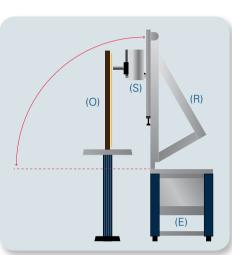
Diagram of the M6 JETSTREAM set-up in the upright measurement position, showing analysis object (O), spectrometer head (S), rig (R) and electronics compartment (E)
