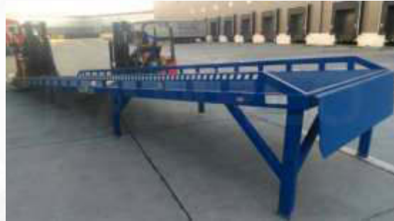
Fixed loading ramps without horizontal boards
