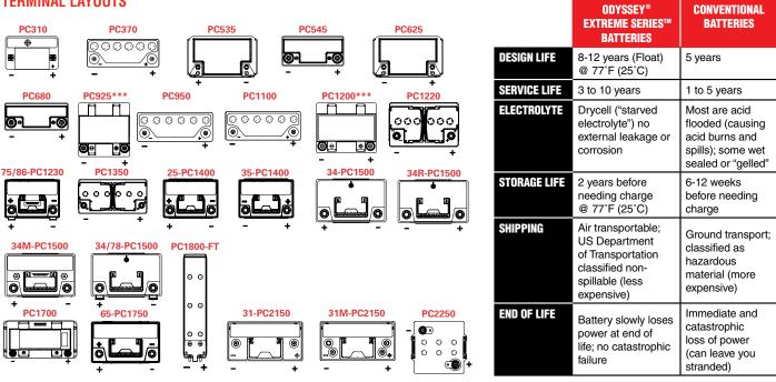
Drawing sizes are for terminal position reference only; diagrams are not proportionate to each other.
