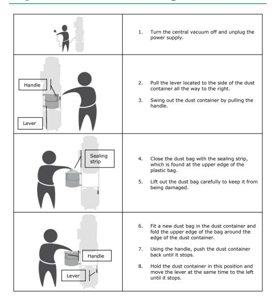
The dust bag might contain hazardous and poisonous dust and should therefore be disposed off according to governmental regulations. Used dust bags should always be closed completely and be treated carefully. Use only original dust bags.
