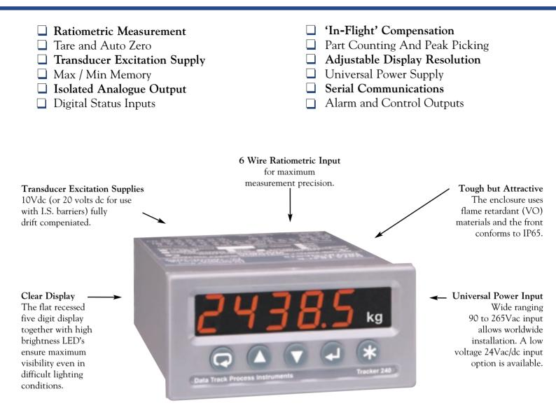
The Tracker 240 series of digital panel indicators are designed specifically for use with load cell transducers and for weighing applications. All the Tracker 240 series models have a 5 digit display and transducer supply plus many software features including tare, offset zeroing, 'in-flight' compensation, 'peak picking' and extensive alarm functions.
