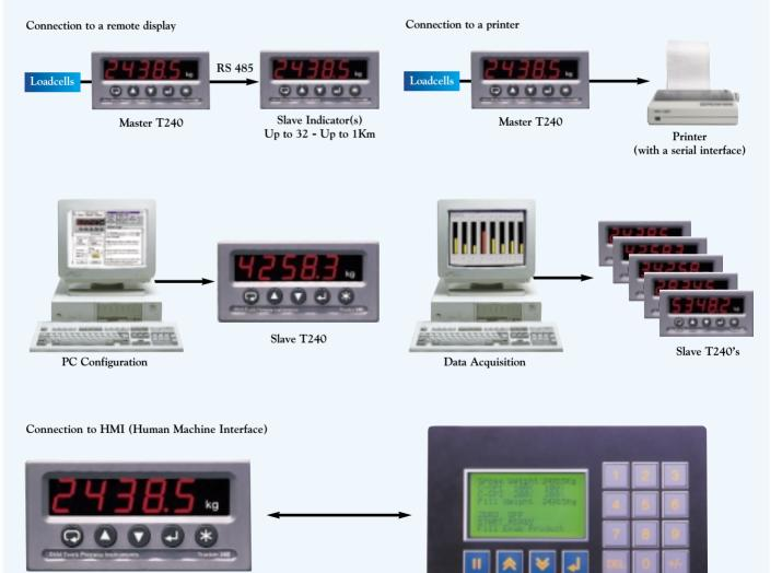
The combination of a Tracker 240 and an HMI, fitted with a Modbus compatible RS485 interface, becomes a powerful stand-alone batch control system and recipe selection system. The HMI's display and function buttons can be tailored for any application and language. Many HMI units can also be a gateway for Fieldbus connection (e.g. Profibus, Device Net). A single HMI can communicate with up to 32 Tracker 240 units.
