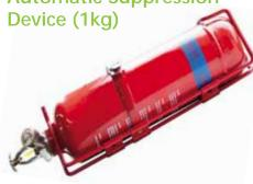
Glasdon FireSafe automatic fire suppression device is fitted within the hood of the bin. Should a fire break out inside the bin the device is activated. Glasdon FireSafe is an effective low cost auxiliary device and must never replace primary fire prevention measures. A regular inspection/maintenance programme should be introduced to ensure the device is in working condition or has discharged and therefore needs replacing.
