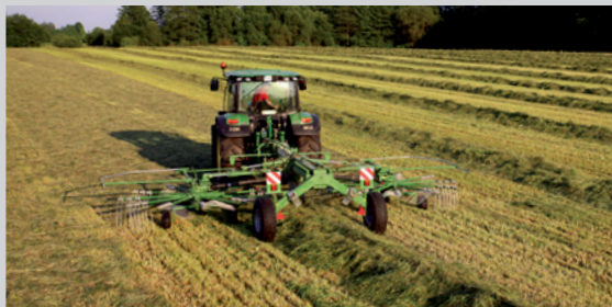
SIPMA ZK 650 WIR RAKE THANKS ITS SPAN ALLOWS RAKING LARGE ACREAGE IN A SHORT TIME
