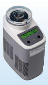
The electronic water bath thermostat with Peltier element is a versatile and powerful device used to control the temperature of refractormeters, polarimeters etc.
