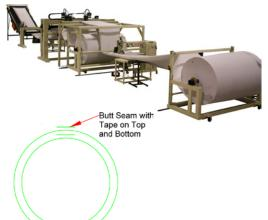
The Miller Weldmaster automatic tubing system is able to pull non-woven fabric off of roll, pre-fold into a desired tube diameter and sewn into a tube. After the system has sewn the system then welds a tape over the sewn seam. The cured in place tube is then wound up on a core as a laser writes a programmed company name on the tube. The filter tube system has line speeds up to 60 feet per minute with limited to no operator involvement.
