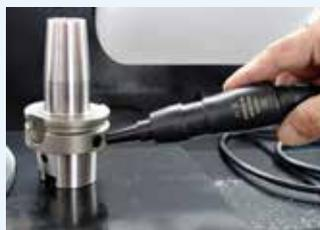
**BIS-C Chip Reader** BIS-C Chip Reader
