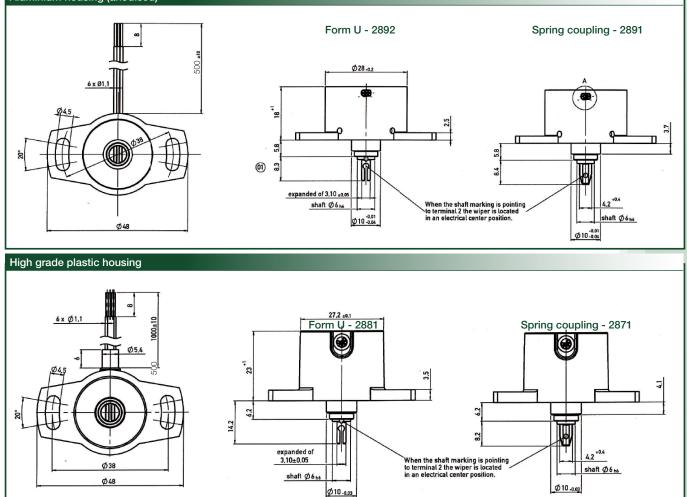
Form U and Spring coupling shaft detail for both housing types
