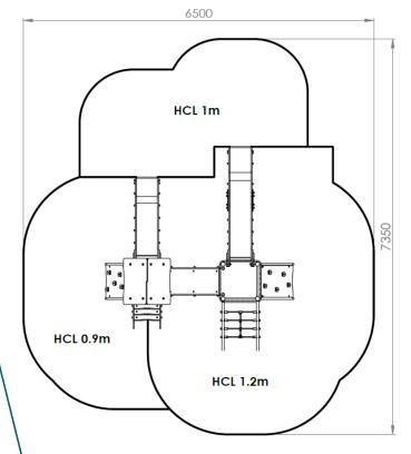
HCL 0.9m: 9.1 m<sup>2</sup> HCL 1m: 8.4 m<sup>2</sup> HCL 1.2 m: 19.2 m<sup>2</sup>
