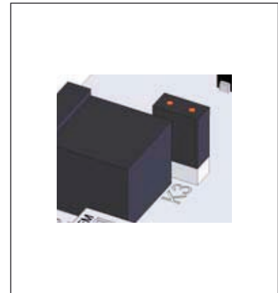
Fig. 31: Plug-in jumper K3 ON
