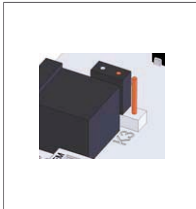
Fig. 30: Plug-in jumper K3 OFF
