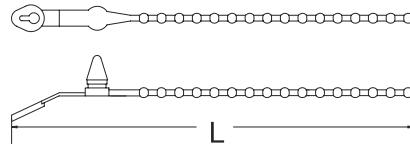
Material: UL approved NYLON 66, 94V-2. Easy to install and release. Beaded design keeps wires from shifting or slipping.
