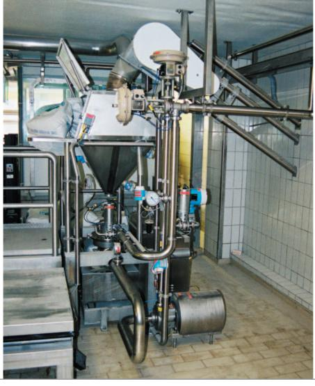
YTRON-XC with bag-emptying station Application: Production of Concentrates prior to Spray Drying
