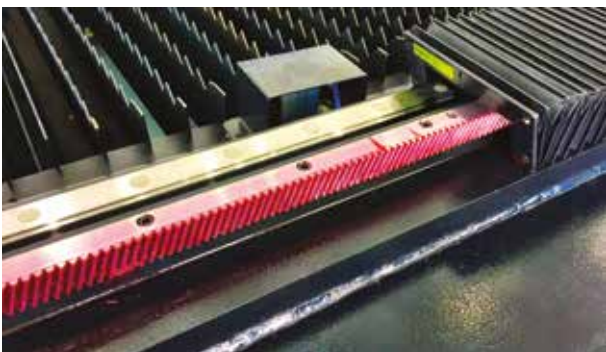
Linear axis with double pinion and rack drive.
