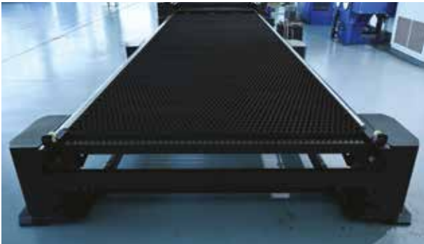
Automatic pallet changer for continuous operation.
