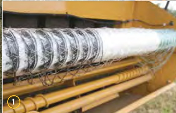
1 The 5520 features an optional netwrap system that makes net convenient to feed and operate. No more hassles or confusion with belts and rollers. Just feed the net directly to the baler's main belts and spread net to the edge of the bale.
