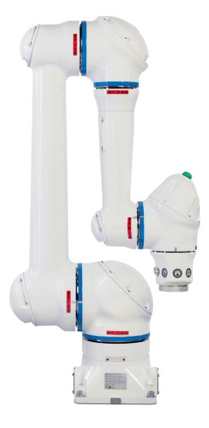
MOTOMAN HC10DT IP67 (B10 + B12) are 6 axes human-collaborative robots with a payload of up to 10 kg. Complying to EN 60529-IP67, they are dust and waterproof protected to operate in harsh environments. Operator's safety is assured by a Power and Force Limit technology that stops the robot in case of contact with an operator.
