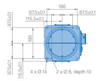
Mounting options: Floor, ceiling, wall, tilt\* Protection class: EN 60529-IP67
