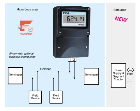
The BA414DF Fieldbus Indicator is a new cost-effective intrinsically safe field mounting instrument that displays a single fieldbus process variable in a hazardous area. Housed in a robust IP66 GRP enclosure, the instrument has a large, high contrast five digit display, plus a horizontal bargraph. The BA414DF indicator uses the same technology and compliments the well established BEKA eight variable fieldbus displays that are now in worldwide use.
