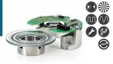
Photoelectric rotary encoder A75M is used to establish an informational link between the key machine components, industrial robots, comparators and DCC, NC or Digital Readout Units. It provides information about the value and direction of the motion. The encoder is used in automatic control, on-line gauging, process monitoring systems, etc.
