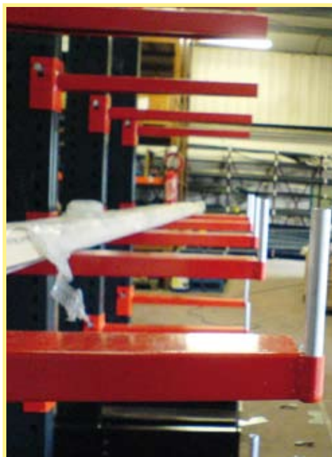
Stockage de charges longues type CANTILEVER
