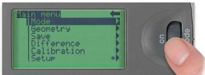
You can select Mode, Geometry selection, Difference, and Calibration from the Main Menu screen.
