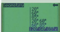
You can select the measurement angle from the Geometry selection screen and display two angles or three angles at the same time.
