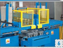
To load the longitudinal elements into the guiding channel, machine can be endowed with automatic feeders to feed the elements out of a special hopper where elements are stacked. duplex feeder can be placed on the right and/or left of the machine's main belt. Each duplex can feed max. 3 guiding channels.
