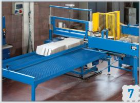
After assembly, partitions can be collapsed (automatically folded flat), counted and divided into batches and delivered onto a delivery table ready to be packed by means of the collapser automatic delivery device (optional).
