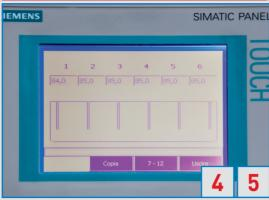
The machine is controlled and operated from the touch screen panel installed on electrical cabinet. From this HMI the operator processes and save data related to the different partitions like: number of cuts in longitudinal element, motors speed, injection timing, etc
