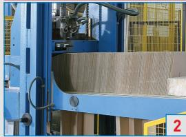
Cross dividers feeder is built on the top of the interlocking area, in the middle of the machine. The elements are kept upright by a pressure system and moved to the injection area by means of belts.
