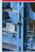
Once the longitudinal elements r are detected from a photocell which that pushes cross elements throu ensure a precise penetration of cr dinal ones.
