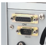
Upper: D-SUB connector Under: RS-232C
