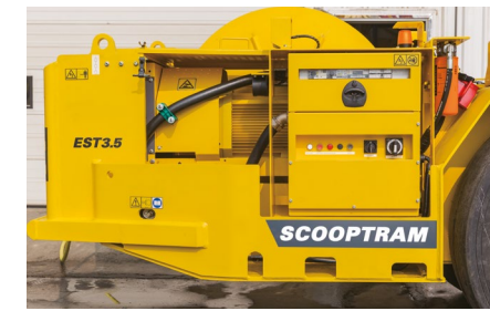
Ground fault and ground check systems are installed to ensure personnel safety.
