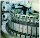
Using the scrip wheel you bring the flash frequency of your rolux into alignment with the movement frequency of the knitting mackine. The excellent illumination of the measuring surface and the imaging, which slows down the sequence of movements, now allows you to check that guides, rollers and needles are working.
