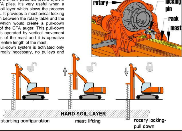
MULTI-PURPOSE DRILLING RIG
