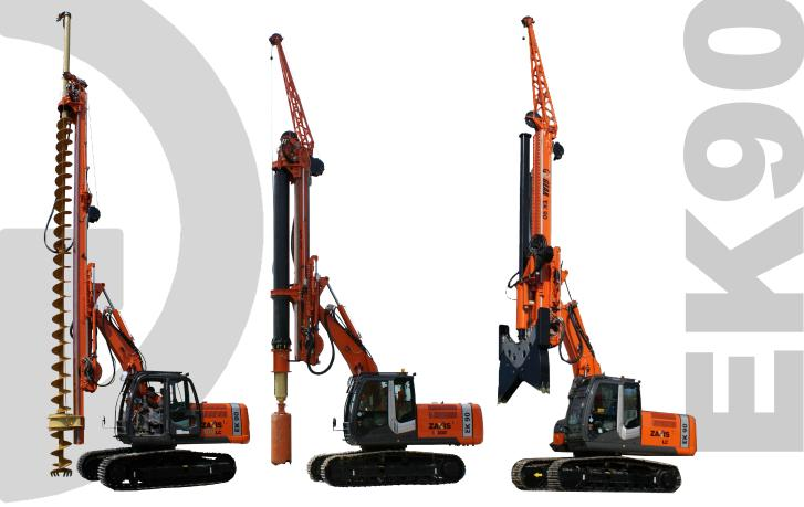
GEAX EK90 (as all the other GEAX machines) is characterized by an articulation architecture similar to a normal excavator, with a long boom in which is attached the mast. This permits a wide range of mast positioning and independent movements for the vertical alignment. Rope paths do not depend on the position of the mast since winches are fixed on it. This architecture, compared with that (usually parallelogram) of other machines, ensures:
