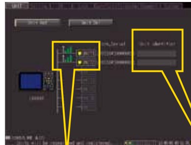
You can verify if the communications state between the LR8410-20 and detected units is good.
