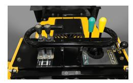
**ENJOY THE RIDE.** A dedicated rubber-mounted operator platform integrates an operator presence system and helps keep the operator out of the mud. The intuitive controls include dual, single-axis joysticks for precise ground drive control which helps in maintaining a straight trench. The ride-on platform enables easier cross trenching.
