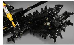
ADJUST YOUR TRENCH WIDTH. The FTX25 uses welded cutter spacers making it easier to change from 8", 10" or 12" (20.3 cm, 25.4 cm or 30.5 cm) cutting width and back without having to remove several spacer blocks.
