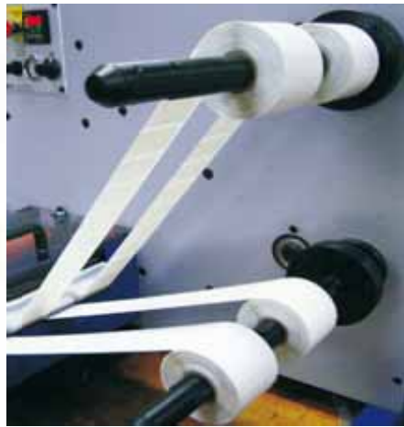
Twin rewinds (air shafts)
