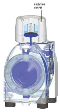
Due to their design, pumps with oscillating action produce a pulsating flow. Although the double-acting design of the E-Series and the direct pneumatic drive have already greatly reduced the pulsation, a pulsation damper must still be installed on the delivery side in order to obtain a virtually uniform flow.
