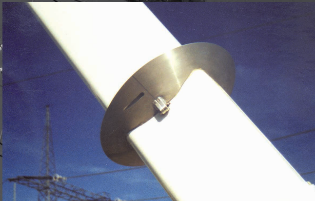
A sharp-edge corona ring provides a consistent voltage gradient along the length of the FRP boom.
