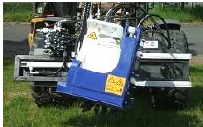
EX 30 Standard Patch Planer mounted on Loader Frame with Hydr. Side Shift and Swing Device
