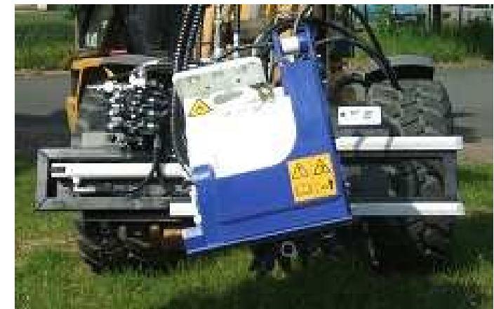
EX 30 Standard Patch Planer mounted on Loader Frame with Hydr. Side Shift and Swing Device
