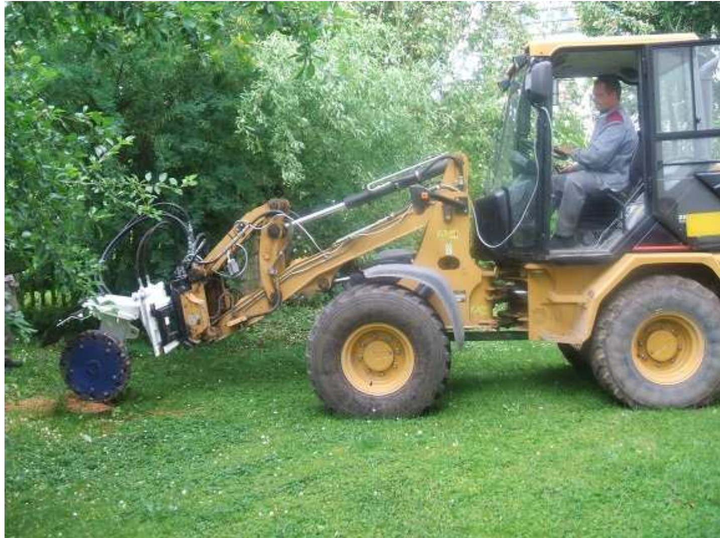
EX 30 Standard Wood Cutter with Hydr. Side Shift and Swing Device Mounted on Articulated Wheel Loader
